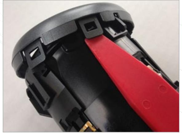
**2** Release the final clip connecting vent fascia to the vent housing.
