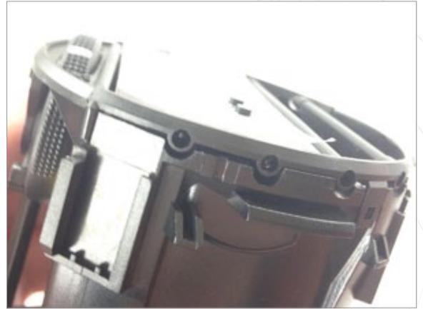
**10** Reinstall the horizontal slat retainer assembly with the VIDI now installed.
