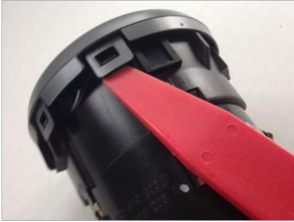
**1** Release the clips on connecting the vent fascia to the vent housing.
