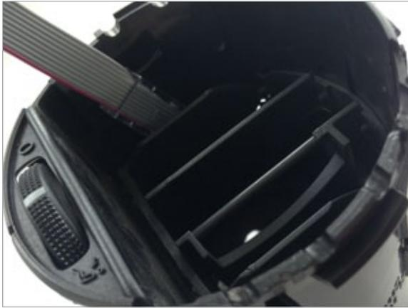
**9** Feed display cable in on far left side of vent between the vent wall and the last vertical slat.
