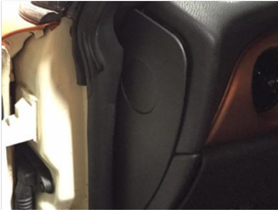
**1** Using your finger or a soft trim pry tool open the side dash cover panel.
