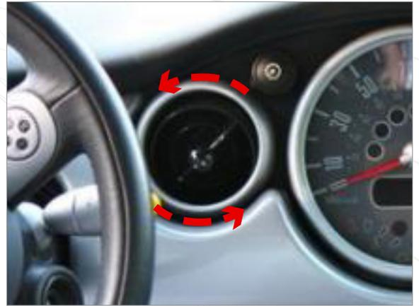
**2** Twist to release the silver appearance trim ring. Use a gentle twisting to the left motion as shown.
