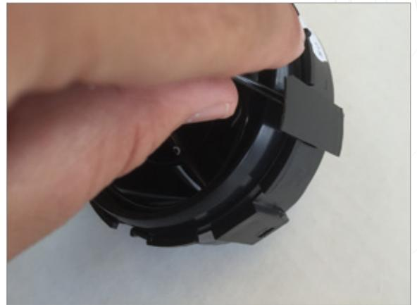
**6** While holding the clip down with your small flat head screw driver insert a shim between the clip and the dash.
