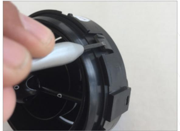
**4** Slide a very small flat head screw driver in the middle of each tab where it is open and between the two grab clips that are on each tab as shown.
