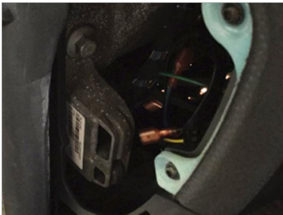
**10** Tuck control box and wiring snugly in the side dash area who's panel you removed in step one.
