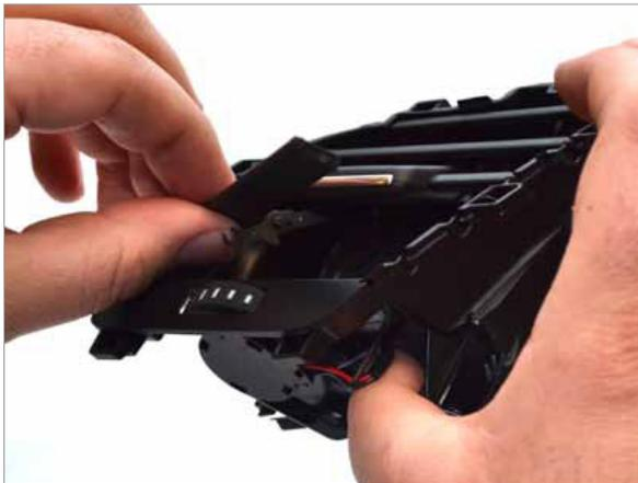
**5** Now remove the second from bottom slat, this slat will have a small metal controller bar behind it that will need to unhook from the slat above it as it comes out. Once again, take care that the other slats do not come out.
