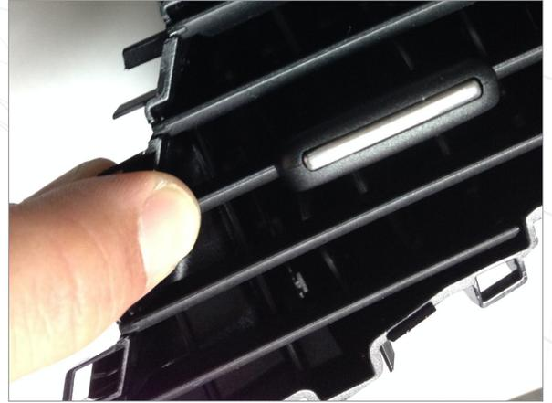
**2** Place index finger over the central control slat while removing lower slats. This will insure control and upper slats remain in the vent and in union with one another.
