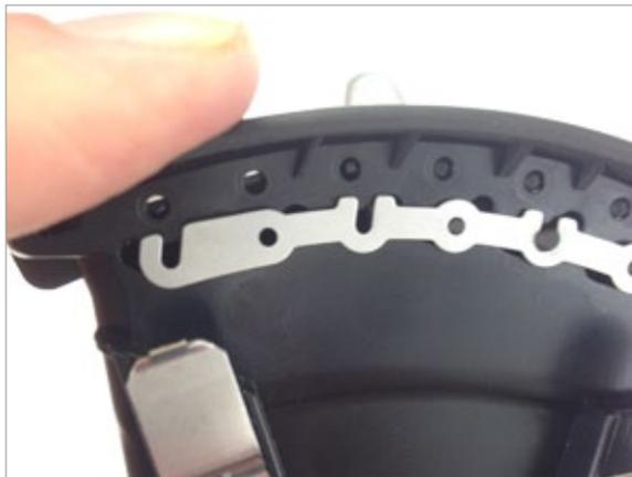
**16** Ensure the right side of Facia makes positive contact and clips into place.
