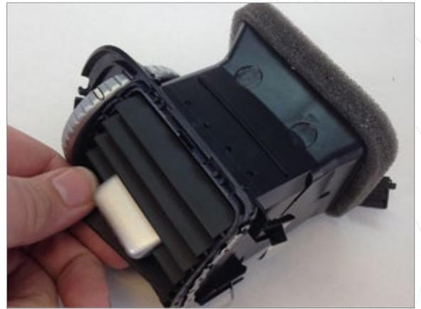
**10** Remove the bottom horizontal vent slat.
