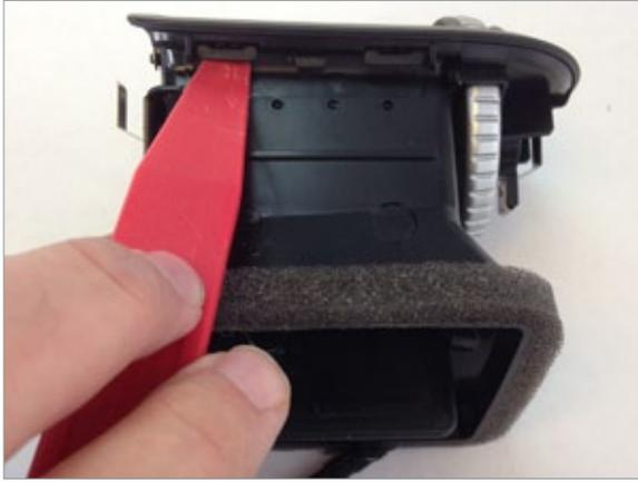
**1** Starting on top of the vent release the left most tab connecting the Facia trim to the vent housing.
