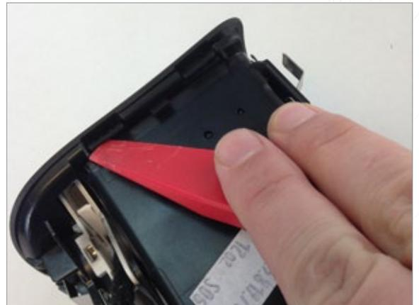
**6** Release the final clip connecting the Facia trim to the vent housing.
