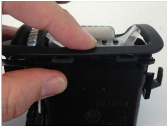
**14** Starting at the bottom of the vent reattach the Facia trip. Ensure the VIDI's protective covering does not get pinched. This will prevent you from being able to cleanly remove the protective covering.
