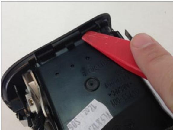
**5** On bottom of the vent housing release the right most clip.
